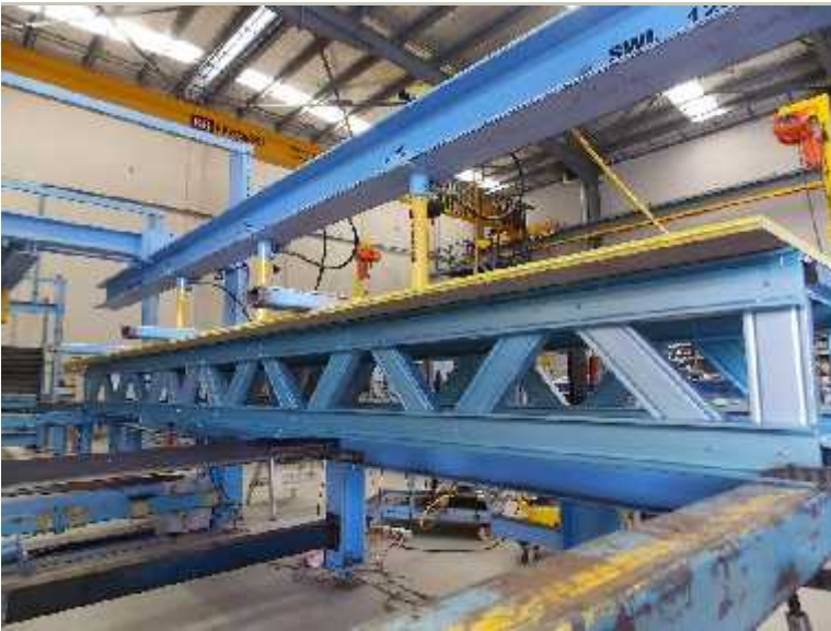
The ENDUROFLOOR™ system being tested by Lysaght® Research & Technology (LR&T)
