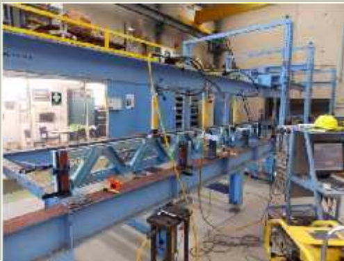
The ENDUROFLOOR™ system being tested by Lysaght® Research & Technology (LR&T)
